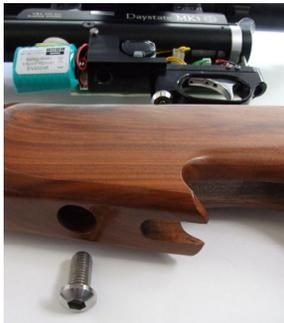
3. With the stock removed, locate the trigger pivot pin and remove. This should only require light pressure or can be gently assisted.
