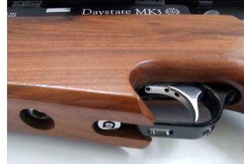
2. Ensure the electrical isolation switch is set to safe with the key. Remove the stock retaining bolt from the bottom of the stock with an 8mm allen key and withdraw the stock from the rifle.
