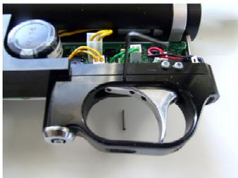
4. Gently ease the original trigger out of the guard.
