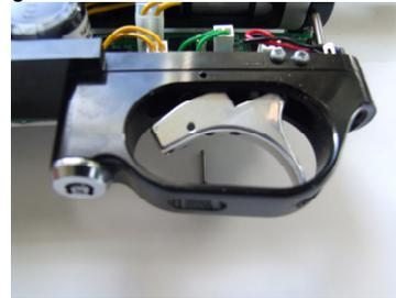
5. Take the spring and cap out of the original trigger and put them in the replacement trigger. Visually match the grub screw settings across to the new trigger. Loosely set the trigger post to the position of the original trigger to assist assembly. Do not tighten.
