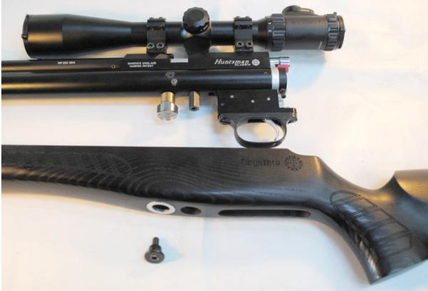
3. With the stock removed, remove the trigger guard and press out the trigger pivot pin. This should only require light pressure or can be gently assisted. Take care not to allow the other pins to drop from the mechanism.
