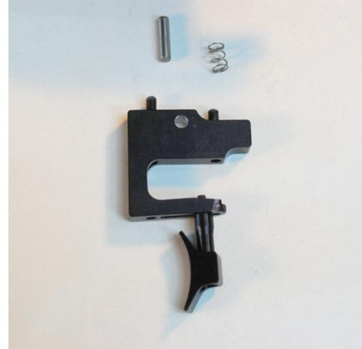
5. Take the spring from the original trigger and locate on the replacement trigger. Visually match the grub screw settings across to the new trigger. Loosely set the trigger post to the position of the original trigger to assist assembly. Do not tighten.
