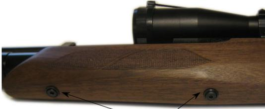
Remove 2 stock retaining screws.
