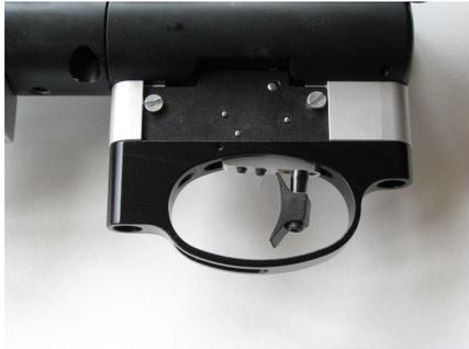
Refit trigger guard and cover plate
