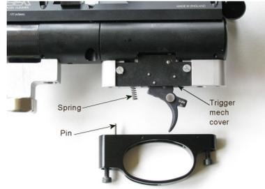
Remove trigger guard retaining screws.
