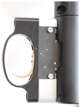
Refit trigger guard and cover plate
