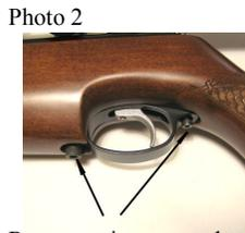
Remove trigger guard retaining screws.
