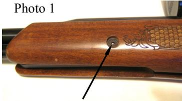
Remove countersunk screw from both sides.
