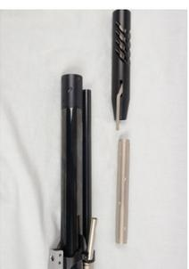
4. Lightly oil or grease the barrel. Take the shorter sleeve and slide it on to the barrel.
