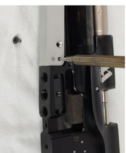
3. Remove the factory airstripper and front aluminium sleeve.
